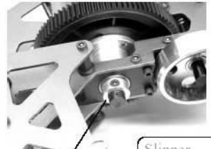
#HW6054 Bottom Collar & M3x6 Flat head screws x 2
